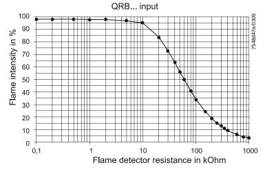
A flame detector resistance of RF <500  $\Omega$  is identified as a short-circuit and leads to safety shutdown in operation, like in the case of loss of flame.
